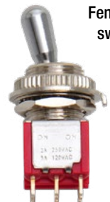
EL02M Mini Toggle Switch, on/on, chrome. Compact toggle switch with 2 x 3 solder pins. Usable as a pickup on/off switch, a coil tap switch or similar.
