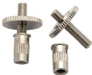
HW4RN Tunomatic Height Adjuster Wheels, 1pc nickel. Instead of turning the knurls, take a 2mm allen wrench from top. Bushings Ø6mm, 11mm long.
