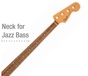
099-0226-921 '60's Jazz BASS C Neck, 20 Medium Jumbo Frets, Maple, Road Worn Nitro finish, 9.5" radius Pau Ferro fingerboard, Vintage-style truss rod adjustment.
