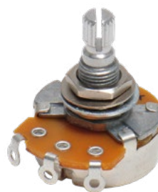
EL500 Deluxe Pot, heavy duty, 8mm, 500K log. Threads 10x8mmØ, housing 24mmØ, knurled shafts. Smooth-running, tin plated housing for easy soldering!
