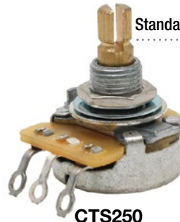
CTS250 Original CTS Push/Pull Pot, 250K log. Made in USA. Threads 9x10mmØ, housing 24mmØ, knurled shaft.
