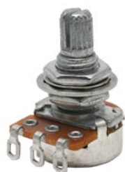
EL25K Mini Pot, heavy duty, 8mm, 25K log. Small size. Threads 10x8mmØ, housing 16.5mmØ, knurled shaft.
