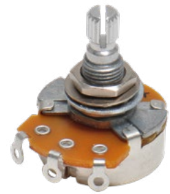
E250L Deluxe Pot, heavy duty, 8mm, 250K lin. Made in Japan. Threads 10x8mmØ, housing 24mmØ, knurled shafts. Smooth-running, tin plated housing for easy soldering!
