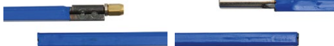
WS40G Double Trussrod, 440x6x9mm. A round and a flat rod, soldered to- gether at one end, one tightening against the other. 7mm nut, US threads. Weight: 164g.
