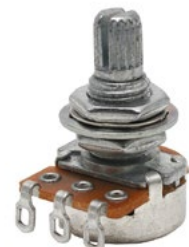
EL1MG Mini Pot, 1M log. Small size. Threads 10x8mmØ, housing 16.5mmØ, knurled shaft.
