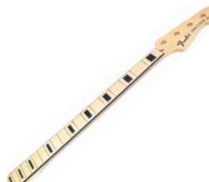
099-2010-921 Classic Series 70's Precision BASS C Neck, 20 Med. Jumbo Frets, Maple with walnut «skunk» stripe, finished, 9.5" radius, 34" scale, pre-slotted nut, block inlay.
