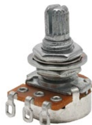
E500M Mini Pot, heavy duty, 8mm, 500K log. Small size. Threads 10x8mmØ, housing 16.5mmØ, knurled shaft.
