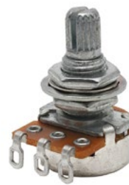
E100M Mini Pot, heavy duty, 8mm, 100K log. Small size. Threads 10x8mmØ, housing 16.5mmØ, knurled shaft.
