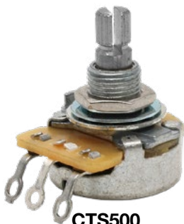
CTS500 Original CTS Pot, 500K log. Made in USA. Threads 9x10mmØ, housing 24mmØ, knurled shaft.
