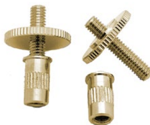
HW4RG Tunomatic Height Adjuster Wheels, 1 pair, gold. Instead of turning the knurls, take a 2mm allen wrench from top. Bushings Ø6mm, 11mm long.
