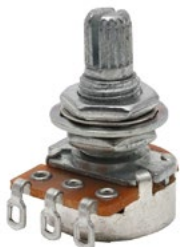
E250M Mini Pot, heavy duty, 8mm, 250K log. Small size. Threads 10x8mmØ, housing 16.5mmØ, knurled shaft.
