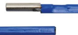
WS41G Dual-Action Double Trussrod. 440x5x8mm. A round and a flat rod, soldered together at one end, one tightened against the other. 4mm hex nut. Weight: 116g.
