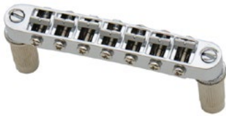
HW27C 7-string Tunomatic Bridge , chrome. With M8 posts. String spacing 62 mm, post spacing 83,5 mm.
