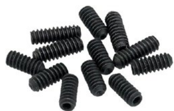
099-4927-000 American Series Bridge Saddle Height Adjustment Screws , black. Set of 12 hex set screws. 4 long (5/16"), 8 short (1/4"). For American & Am. Standard Strat & Tele (1986-2007).
