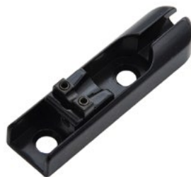
HW60B Bass Bridge 1-string Unit , black. Housing made of zinc, brass saddles. Dimensions 60mm x 15.4mm, string spacing at the bridge min. 15.5mm.
