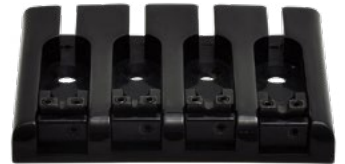
HW50B 3-D Bass Bridge, 4-String , black, single coil. Diecasted like a Badass bridge. Steel lockable saddle. Great sound! String spacing 19mm.
