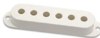
PU01W Plastic Cover for Strat Pickup, white. E' - E string = 52mm / 10,4mm string spacing
