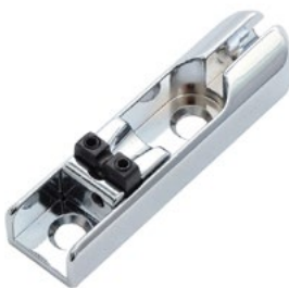
HW60C Bass Bridge 1-string Unit , chrome. Housing made of zinc, brass saddles. Dimensions 60mm x 15.4mm, string spacing at the bridge min. 15.5mm.
