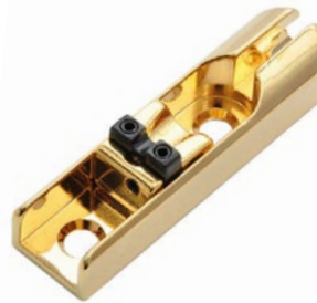
HW60G Bass Bridge 1-string Unit , gold. Housing made of zinc, brass saddles. Dimensions 60mm x 15.4mm, string spacing at the bridge min. 15.5mm.
