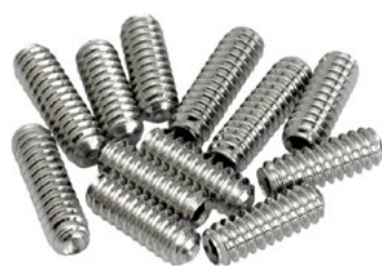
099-4928-000 American Vintage Strat®-Tele® Saddle Height Adjustment Screws , chrome. Set of 12 hex set screws. 4 short (4-40x3/8"), 8 long (4-40x5/16"). For Am. Vintage Strat & Tele.
